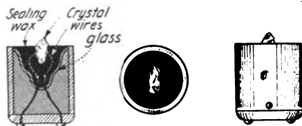
Details of the sealed in detector
