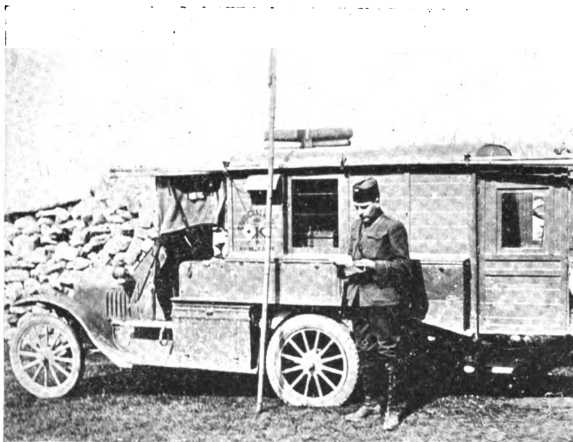
A Ford Tractor equipped with the Divisional Headquarters Radio Set Type E-3 or Type E-3 bis.
