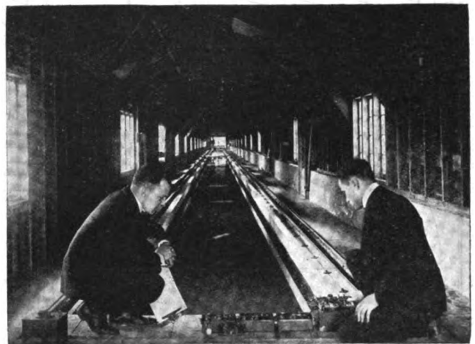
Members of the engineering staff at the research laboratory observing the effects of the transmission of electro-magnetic waves over bare wires laid in fresh water
