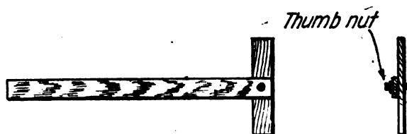
Figure 4—Method of constructing the alidade
