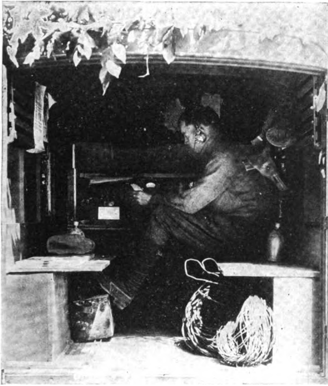
Interior of a Ford Radio Tractor for Divisional Headquarters showing the Radio Set Type E-3 bis mounted therein
